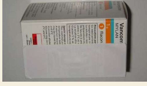
RFID tag attached on powder-based drugs
